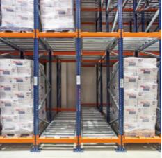
AGILITY AND SAFETY IN OPERATIONS: FORKLIFTS DO NOT HAVE TO ENTER THE RACKS AND ONLY WORK FROM ONE AISLE
