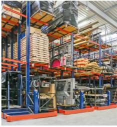
THESE RACKS CAN BE INSTALLED ON MOBILE BASES TO INCREASE STORAGE CAPACITY.
