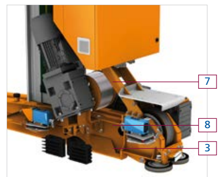
Lower guide base (3), lifting components (7), and rangefinder (8)
